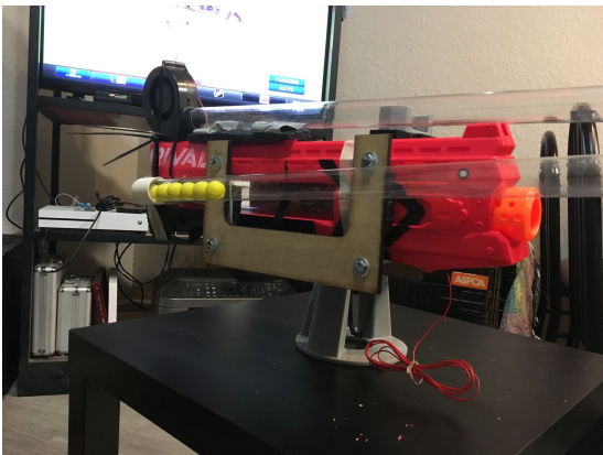
Fig 5. Modification of Rival Zeus model.
